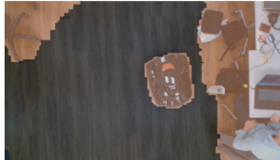
Fig. 12: Realtime test showing the binary prediction as red mask over the input.
