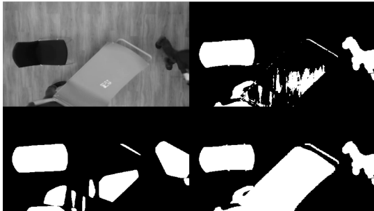
Fig. 5: GrabCut applied on footage (top left: input image, top right: raw 3-channel background subtraction, bottom left: convex hulls created, bottom right: result of the GrabCut filter i.e. produced ground truth).
